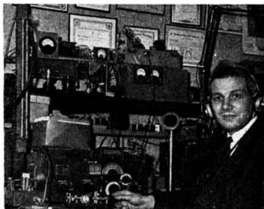
J. Haydon (G3BLP), winner of the I.A.R.U. (Region I) 2-metre Contest, at the operating position. Equipment pictured above from left to right (on shelf)—P.A. unit with 826, exciter with 832 on top of power supply unit; (on table)—2-metre converter, and main receiver (tuning 26–28 Mc/s.). At the extreme left can be seen the 1-wave matching bars (70/300 ohms).
